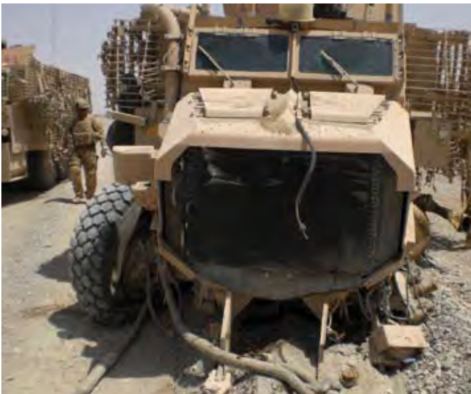
The damage caused by a large IED
